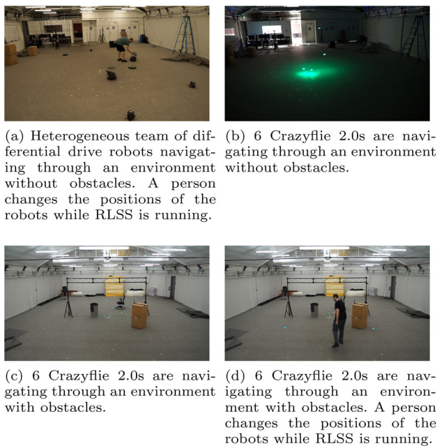
Fig. 9 Physical robot experiments using Turtlebot2s, Turtlebot3s, iRobot Create2s, and Crazyflie 2.0s. RLSS works in real-time under external disturbances
