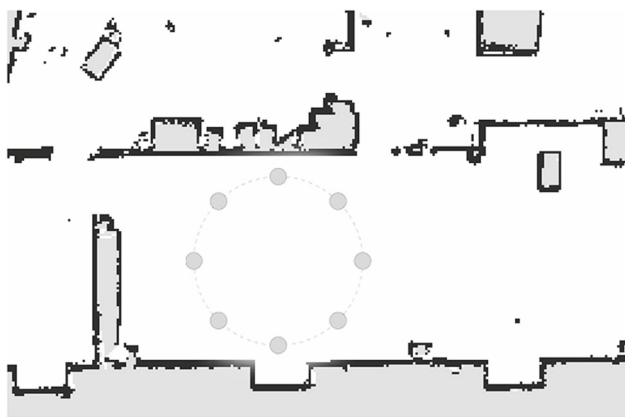
Fig. 15 A sample configuration of the simulation environment for the antipodal circle setting with eight robots
