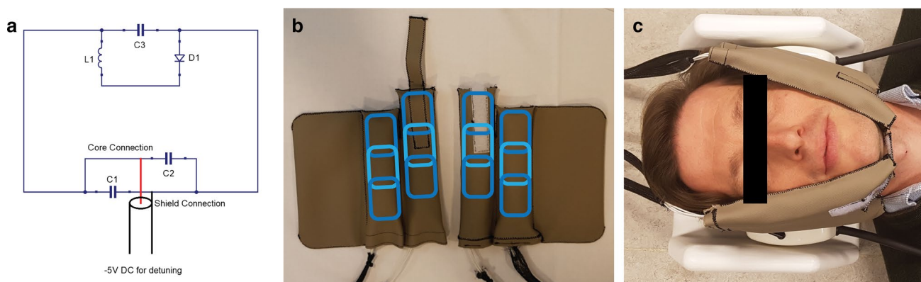
Fig. 1 Design and lay-out of the flexible coil: a the schematic of a single coil element with three capacitors (C1–3), one inductor (L1), and one diode (D1). b Three of these elements were assembled in a phased array indicated by the blue rounded rectangles. c The coil was
