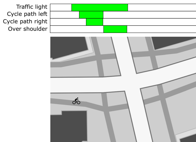
Fig. 2 Example of static MiRA requirements in one intersection located on the experimental route. The intersection consists of two four-lane roads (white) flanked by cycle paths (grey) and pavements. The dark grey structures in the corners are buildings blocking the view from the cyclist's perspective. The green area above the map corresponds to the road stretch within which the cyclist should attend to the respective requirements. Map source: OpenStreetMap contributors (2017) (color figure online)
