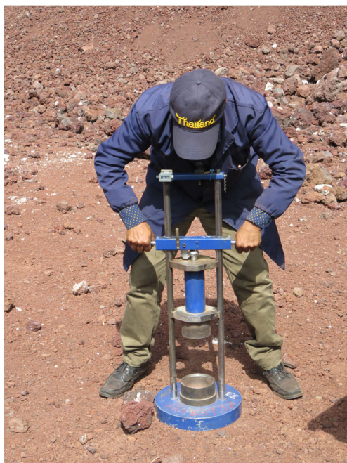
Fig. 10 Site application of the AIV test
