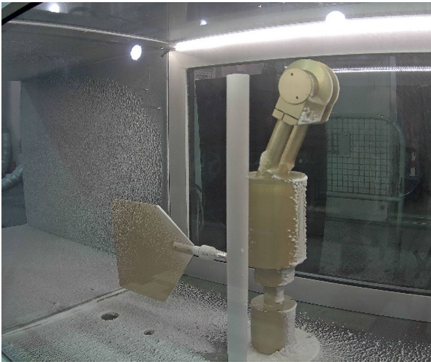
Fig. 12 The image of the ICEMET sensor after the most harsh icing condition test run in the icing wind tunnel at VTT Espoo
