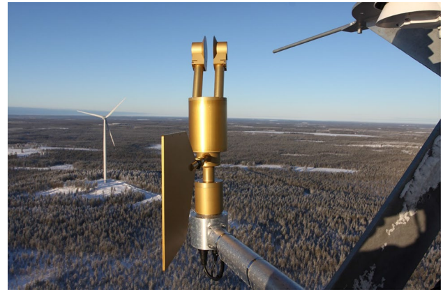
Fig. 13 ICEMET sensor installation on a wind turbine nacelle in 2017
