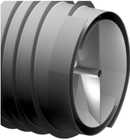
Fig. 8: Side view of the two spiral tunnels beginning at each scoop (without side cover at the scoop side)
