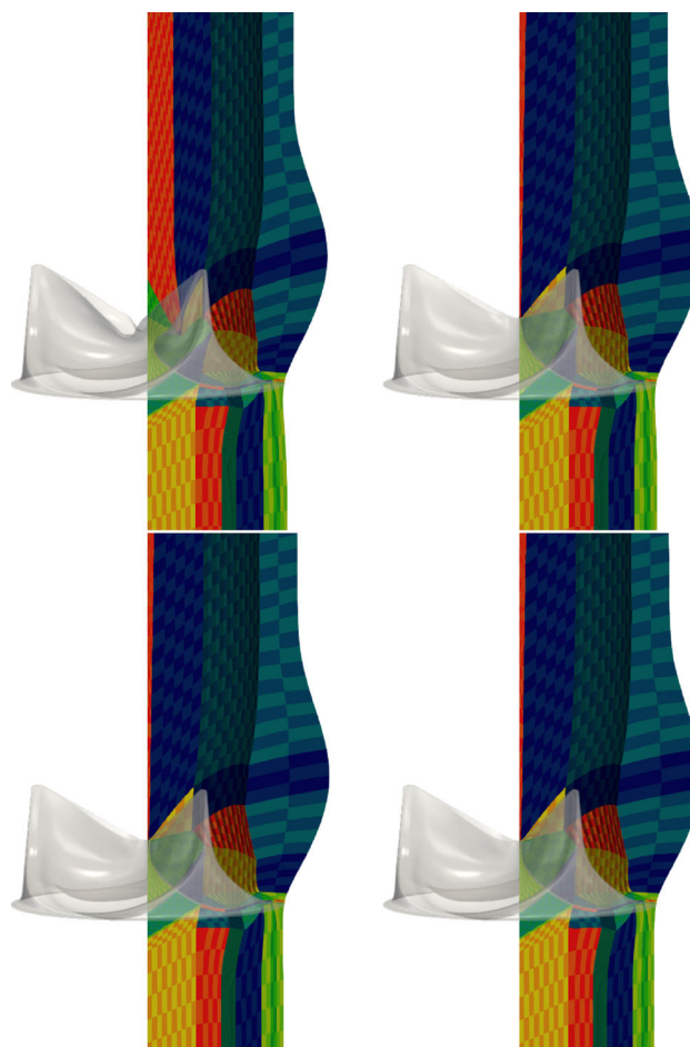
Fig. 9 Cross-section of the volume mesh at t = 0.595, 0.605, 0.635, 0.785 s. The checkerboard coloring is for differentiating between the NURBS elements. (Color figure online)
