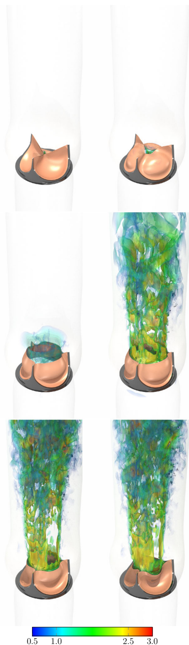
Fig. 13 Isosurfaces corresponding to a positive value of the second invariant of the velocity gradient tensor, colored by the velocity magnitude (m/s). The frames are for t = 1.035, 1.135, 1.175, 1.355, 1.445, 1.450 s
