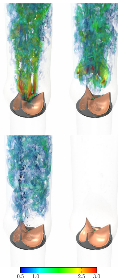
Fig. 14 Isosurfaces corresponding to a positive value of the second invariant of the velocity gradient tensor, colored by the velocity magnitude (m/s). The frames are for t = 1.455, 1.465, 1.495, 1.645 s
