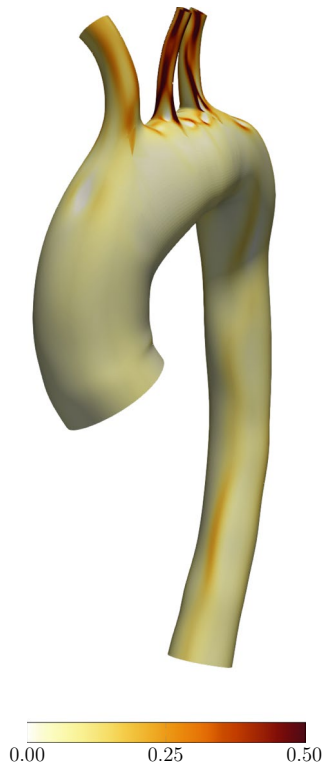
Fig. 17 Patient-specific aorta. \hat{\kappa}_1 ( \text{mm}^{-1} ). The maximum and minimum values are 1.822 \text{ mm}^{-1} and -0.2810 \text{ mm}^{-1}
