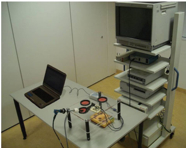
Fig. 2 Testing setup: a box trainer with a target plane (artificial skin pad), TrEndo tracking system, computer used to collect data, and the video system. The cover of the box trainer was nontransparent during performing the tasks
