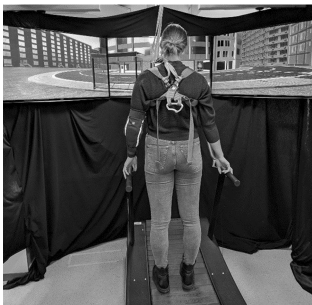
Fig. 1 Setup for the route-finding task. The picture shows a participant on the treadmill, secured by a safety harness, who watches the virtual city on three TV screens
