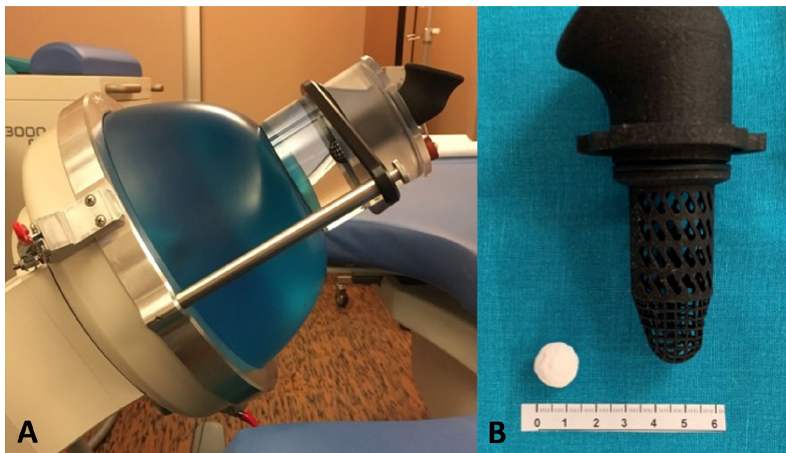
Fig. 1 a SWL-therapy head with mounted test device. b Artificial stone and mesh holder
