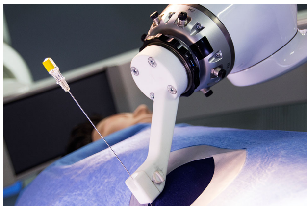
Fig. 2 Guidance tool attached to the robotic arm with inserted needle
