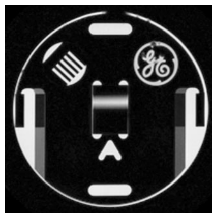
Fig. 2 Axial conventional spin-echo images of a standard S/N and spatial resolution phantom acquired on the OPTIMA MRI scanner demonstrate accurate geometric dimensions and good spatial resolution. Acquisition parameters: TR 500 ms, TE 14 ms, FOV 160 mm, matrix 256 \times 256 , slice thickness 5 mm, receiver bandwidth 32 kHz, number of acquisitions 1, scan time 2 min 8 s
