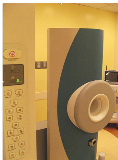
Fig. 1 Photograph of the 1.5-T OPTIMA MRI system after modification for neonatal imaging. Modifications to the OPTIMA system at the time of the sheep studies included increasing the magnet height and leveling to true horizontal. Additional modifications made subsequent to the sheep studies included: (1) replacing the chair used to support the patient for extremity scanning by a customized patient table, and (2) integration of the measurement control electronics, RF chain and system operating software of a state-of-the-art 1.5-T adult-size scanner with the basic OPTIMA system to enable the full spectrum of advanced imaging capabilities. At present, two enhanced neonatal MRI units are installed and in operation at our institution. One system is located in the Imaging Research Center and is being used for preclinical research (such as the initial preterm sheep study). The second neonatal MRI system is located in the NICU and is being used to perform patient examinations and clinical research studies
