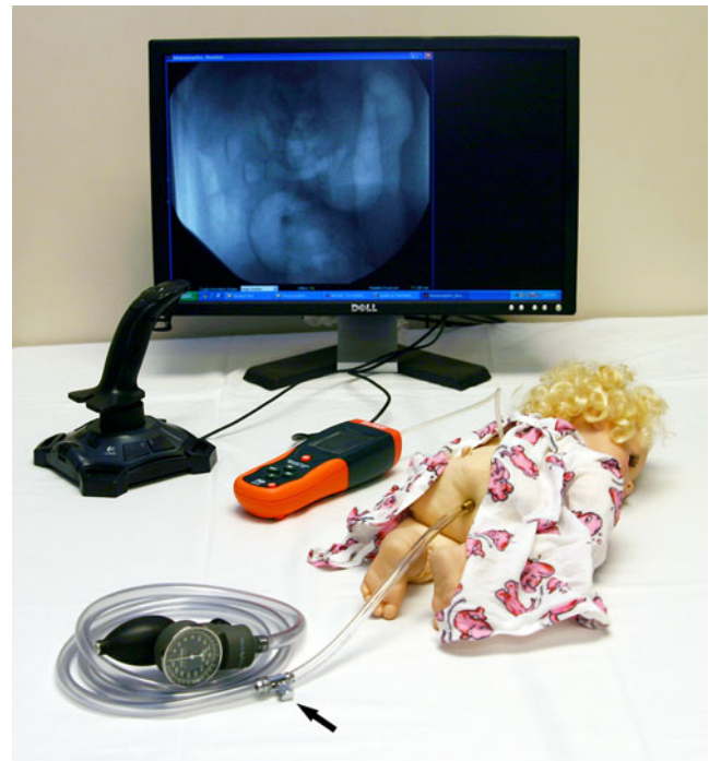
Fig. 1 Plastic tubing with the instructor’s external release valve (arrow) connects the aneroid gauge and bulb insufflator to the cylinder within the doll. Additional tubing extends from the doll to a pressure sensor and is transmitted via USB cable to a computer
