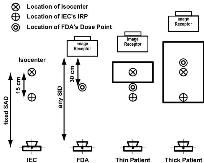
**Fig. 1** Dose reference points. The IEC reference point is defined relative to the isocenter of the imaging system. It is independent of SID. The FDA measurement point is defined relative to the image receptor at any SID. This point moves away from the focal spot as SID increases
