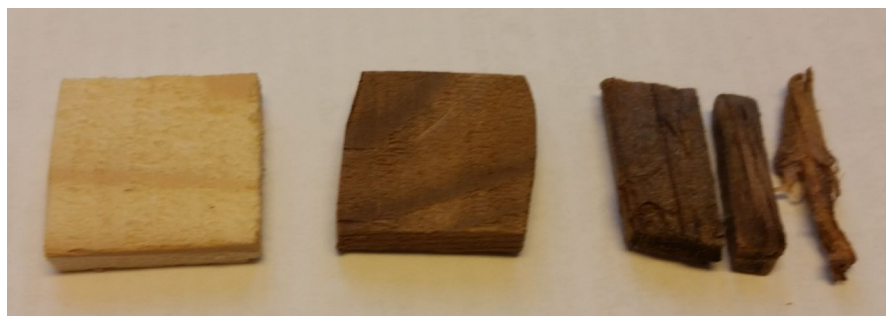
Fig. 1 From left to right: native, SEW, and SEIW. Notice the color change after treatment present for both samples subjected to the steam explosion treatment. Furthermore the SEIW samples show distinct ruptures mostly along the fiber direction (color figure online)
