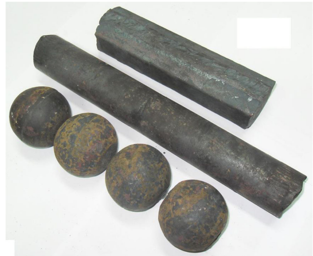
Fig. 14 Starting from top: billet (side-pressed rail head), 52 mm diameter rod, balls with nominal diameter of 70 mm
