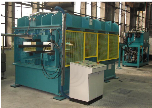
Fig. 12 Flat-wedge reversing mill for producing 70 mm diameter balls
