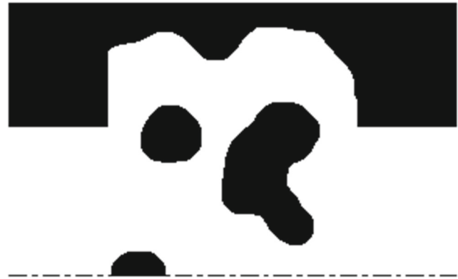
Fig. 3 Waveguide optimized for directional wave propagation from 8–9 KHz
