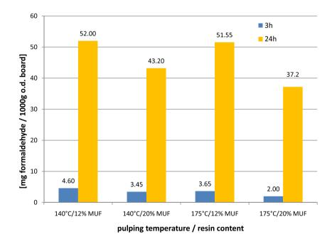
after a reaction period of 24 h. Differences in the formaldehyde release were also registered between the boards made from TMP prepared by pulping wood at 175  $^{\circ}$ C compared to those prepared from TMP obtained by wood pulping at 140  $^{\circ}$ C. However, the influence of resin content in the boards is much more pronounced than that of the pulping temperature.
