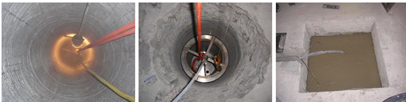
Fig. 17 View into borehole SB2 (diameter 300 mm) after emplacement of sand/bentonite mixture ( left ), after installation of the packer ( centre ), and after grouting of the borehole cellar ( right ) (Rothfuchs et al. 2012)
