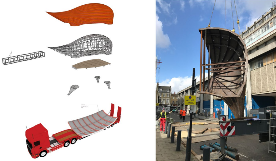
Fig. 13 Diagram of structural components and installation
