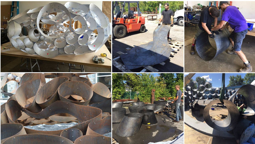
Fig. 7 Fabrication and installation process
