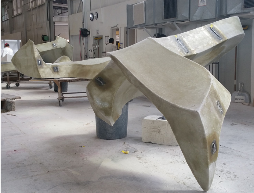
Fig. 22 Corresponding steel connections are laminated onto the matching faces of the parts, allowing them to be joined and carry load in bending
