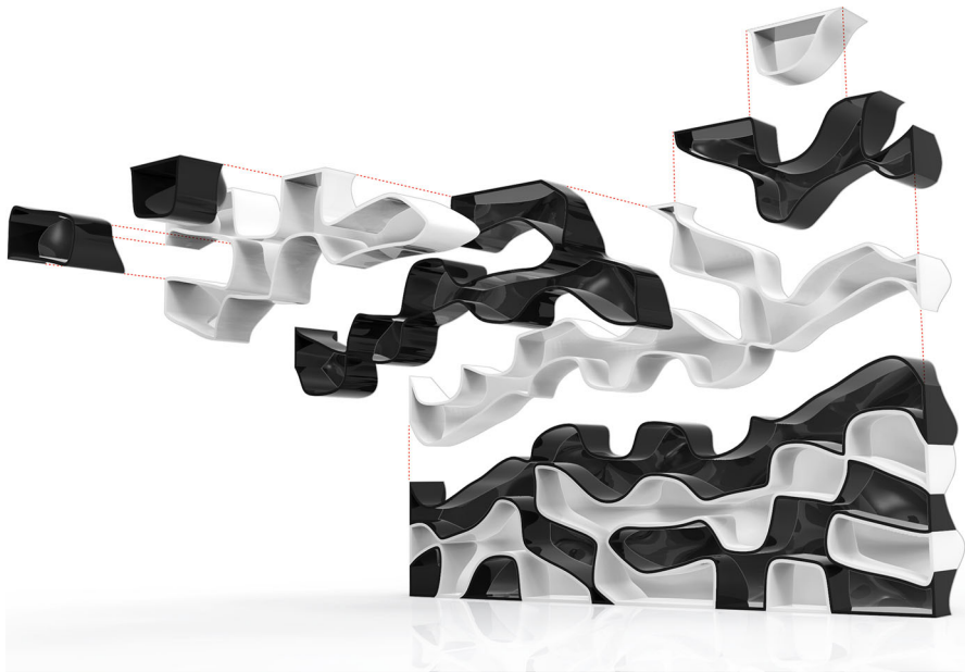
Fig. 4 Stereotomic wall design Type 01 with stacking and nesting parts
