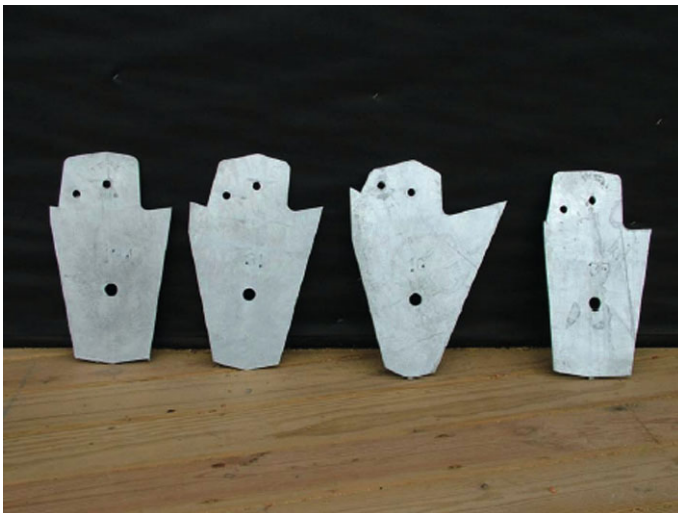
Fig. 1. SHoP Architects: brackets for roof of a post-Katrina hurricane community center, New Orleans, USA. Each piece is an instance of a parametric object defined with the software Catia, using a “Power Copy” command
