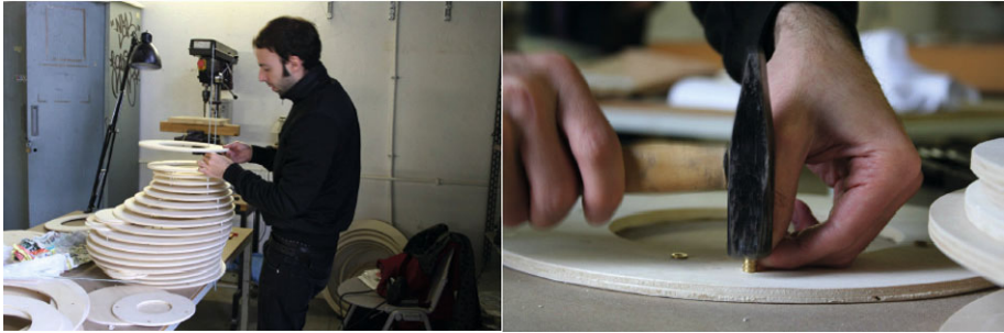
Fig. 13. The assembling procedure of the wooden circles with pre-cut holes
