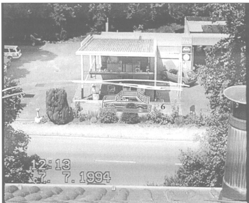
Fig. 8. Estimated trajectories of objects 5, 6, 10, and 11 at half-frame time point #8450. Note that object 6 is leaving the gas station premise beginning with this time point. This is the reason why the front trajectory does not yet extend to the left side of the image frame shown here.
