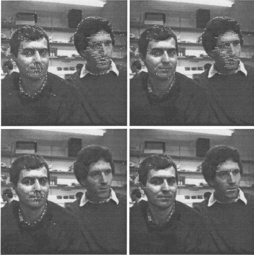
Fig. 3. Showing an image taken from a smoothed sequence of a two heads rotating. The top left image shows the detected feature matches for two images in the sequence. All the points that are tested to see whether or not they are stationary. The top right shows the largest moving cluster detected, the bottom left the next largest cluster and the bottom right the mis-matches.
