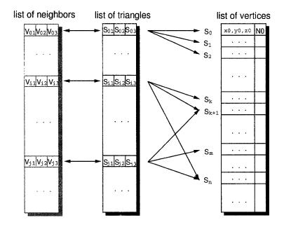
Figure 1: Output data structure of the MC algorithm
