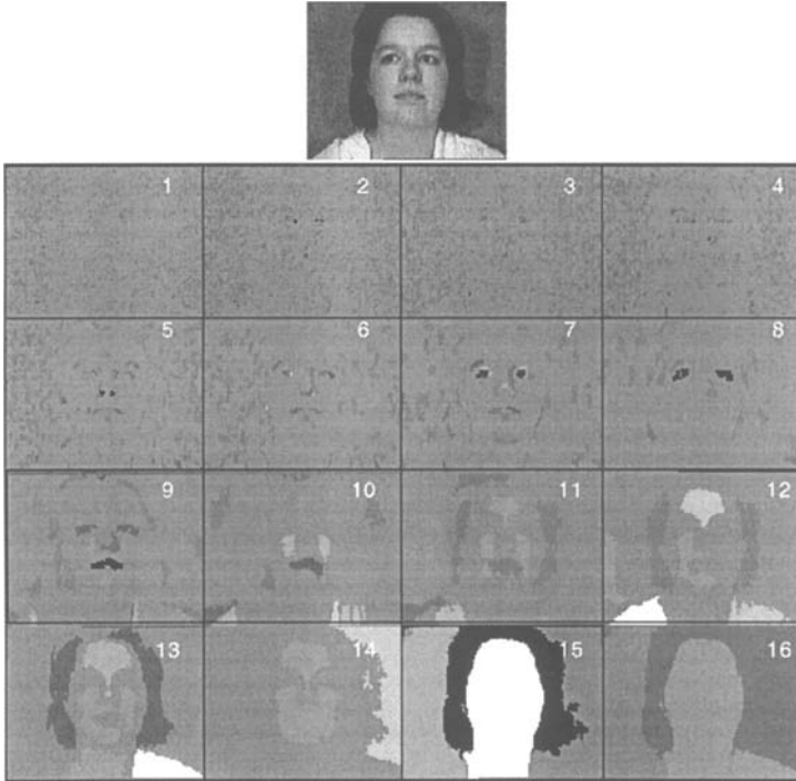
Fig. 3. An area decomposition of an image (top) into a number of channels
