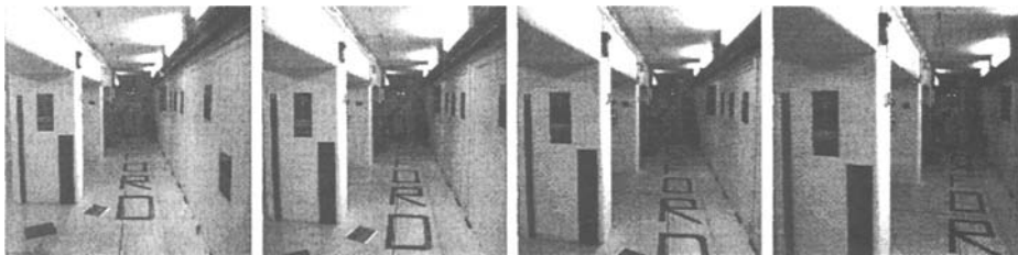
Fig. 4. Image sequence II: four images from a nine image sequence. Planar motion with the rotation axis approximately aligned with the image y axis. 75 corners are automatically matched across the 9 images. The sequence was acquired by a camera mounted on an AGV.
