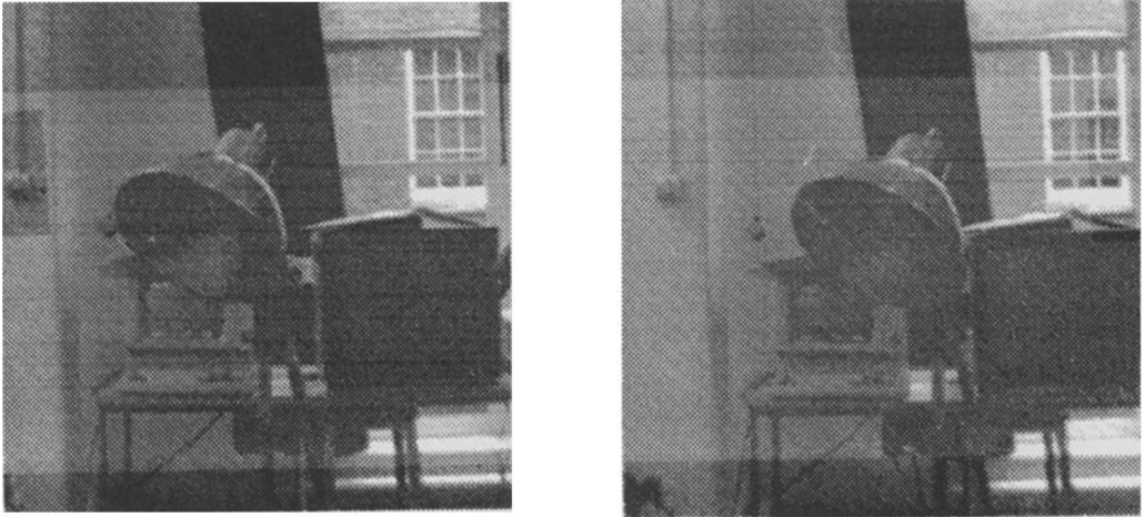
Figure 2: Images taken from a room with a 512x512 CCD camera. Data was compressed to 256x256 using the compact Pyramid. (a) Left image (b) Right image. Disparity differences ranged from 25 (central lamp) to 4 pixels (outside window).
