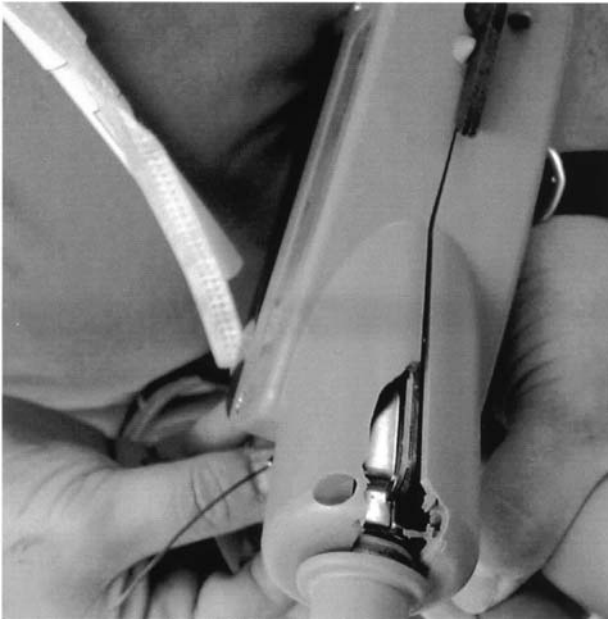
FIGURE 1 Broken transesophageal echocardiography probe connector.
