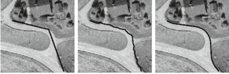
Fig. 10.6 Active contours used to extract roads. Image taken from Laptev (1997)
