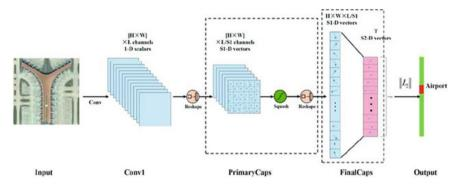
Fig. 9.3 A typical structure of the capsule network (CapsNet) [25]
