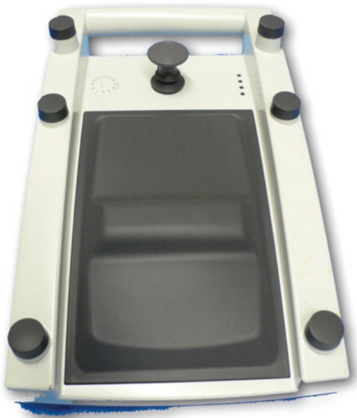
Fig. 30.3 Foot pedal. Foot pedals can serve multiple functions with freely selectable function allocation to several knobs (e.g., photo, video on/off, \pm light, ICG on/off). The joystick steers the microscope head; \pm zoom and \pm focus can be allocated to the left or right side. Wireless function transmission avoids cable clutter
