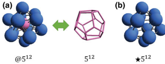
Fig. 6.28 Relation between a local atomic arrangement and a Voronoi polyhedron [12]. a The Voronoi polyhedron associated with the pink atom is 5^{12} . The pink and its neighbouring atoms form a @5^{12} cluster. b The atoms adjacent to the pink atom occupy the vertices of a \star 5^{12} -polyhedron
