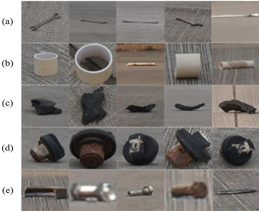
Fig. 3. Examples of FOD images for the classification. (a) Wrench; (b) Plastic pip; (c) Tire debris; (d) Fuel-tank cap; and (e) Metal bar.
