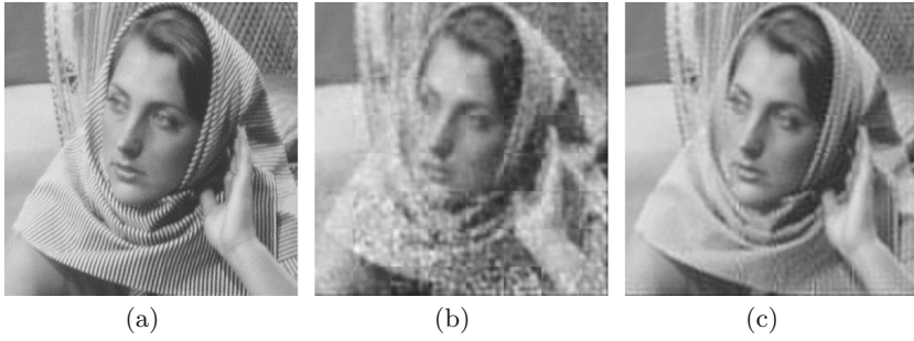
Fig. 6. Test image and reconstruction results of Barbara. (a) the original image (b) the reconstruction result of random Gaussian measurement network (c) the reconstruction result of adaptive measurement network.
