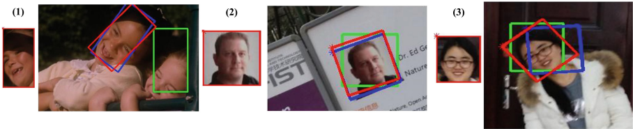
Fig. 6. Template matching results of different rotated template in target image in experiment 2. The green rectangular is BBS's [9] result; blue one is B+S [12] result; red one is ours. (Color figure online)
