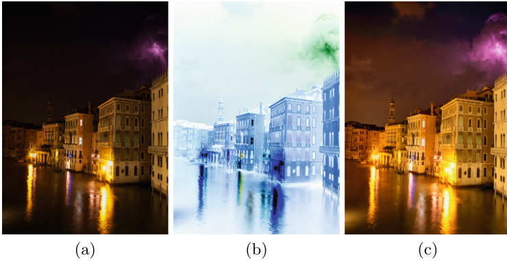
Fig. 2. The enhanced results by our approach. (a) Input low-light image. (b) Inverted image. (c) Image after enhance by our approach.
