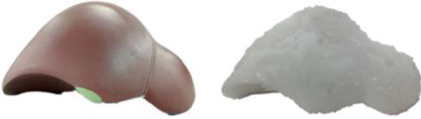
Fig. 4. (a) Liver model, and (b) The phantom of ultrasonic tissue-mimicking materials.
