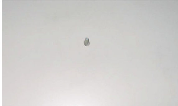
(a) Test hole for measurement of pressure difference
