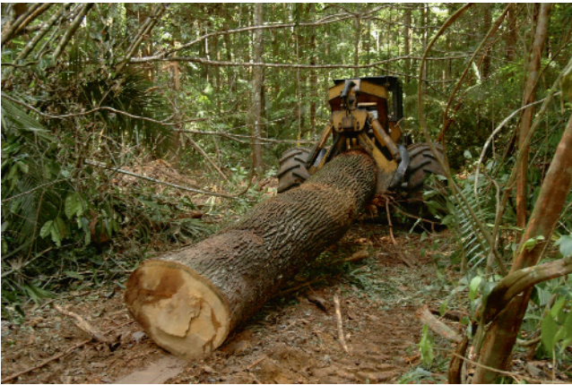
Chapter 5, Fig. 11 Hauling of the logs by driving to the trees using a skidder with a grabber
