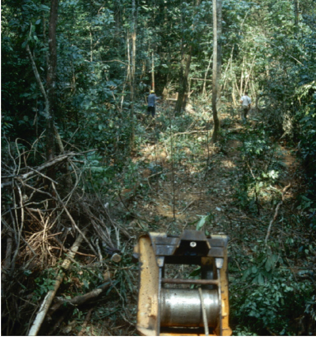
Chapter 5, Fig. 10 Skidder equipped with a winch for cable hauling
