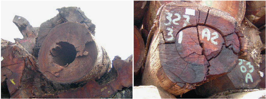
Chapter 5, Fig. 6 Defects of roundwood coming from tropical primary forests
