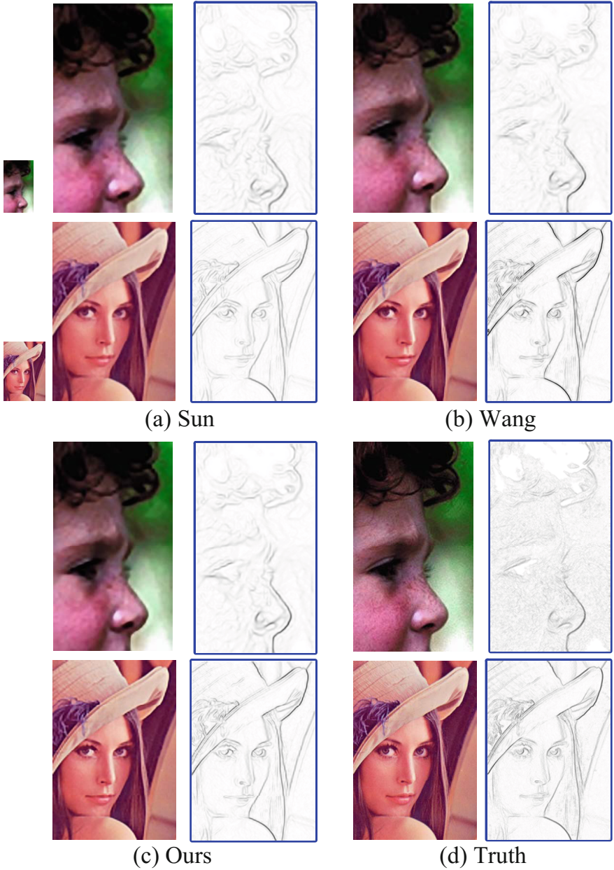
Fig. 4. Comparisons with the edge-directed approaches. The input low-resolution image are the small image in the left. The results of Sun [10] (a), Wang [12] (b), Ours (c) and the ground truth (d). We also present the gradient magnitude of the up-sampled images.
