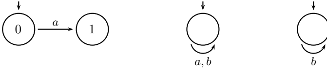
Fig. 3. Processes P_1 with a boolean variable (left), P_2 (middle) and P_3 (right) without variables
