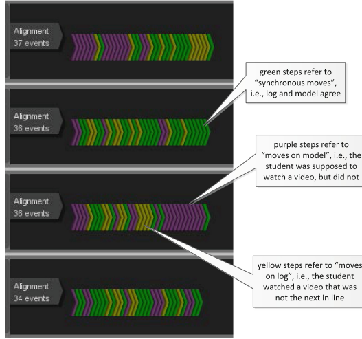
Fig. 3. Alignments for four students showing that few students actually watch the lectures sequentially. The “synchronous moves” show where model and log agree. The “moves on model” show where the student skipped a video lecture. The “moves on log” show where the student watched a video lecture that was not next in line.
