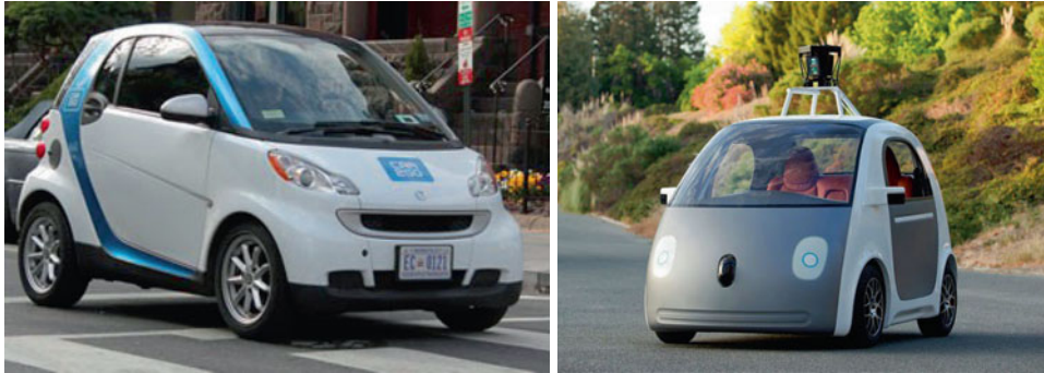
Fig. 19.1 Left figure: A Car2Go vehicle used in a traditional (i.e., non-robotic) MoD system. Right figure: Self-driving vehicle that Google will use in a 100-vehicle AMoD pilot project within the next two years. Image credit: Car2Go and Google.
