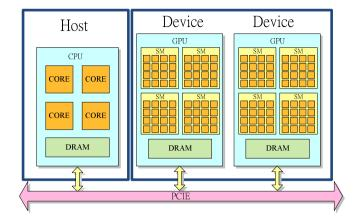
Fig. 1. The organization of a heterogeneous many-core system
