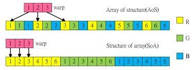
Fig. 2. The data layout of AoS style and SoA style
