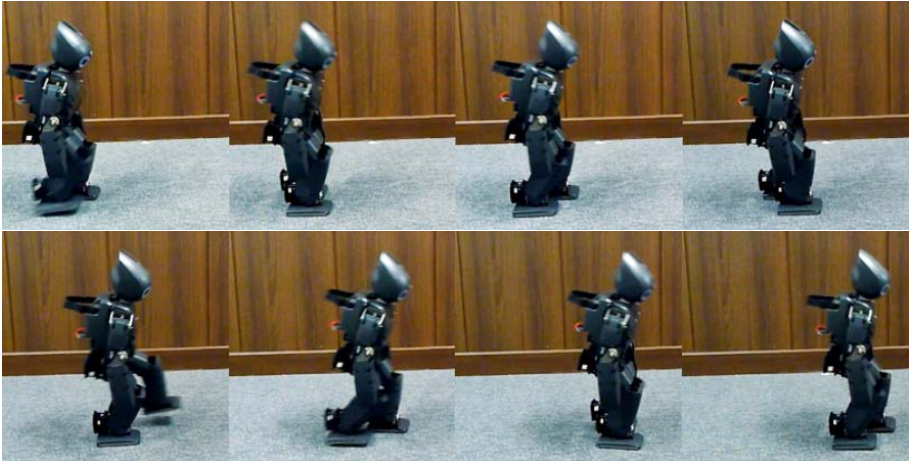
Fig. 2. The ZMP preview control based kick during locomotion
