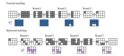
Fig. 4. Recomputations for BKSQ-96 in forward and backward direction.
