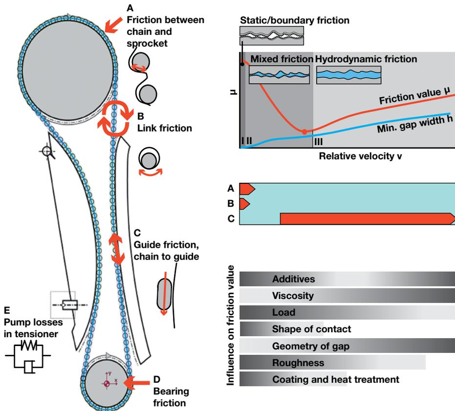
**Figure 11** Friction points in the timing drive
