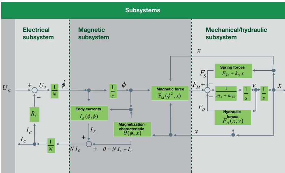
Figure 7 Physical interactions with the quick-acting switching valve
