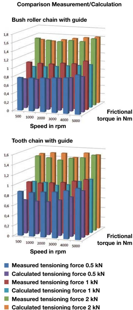
**Figure 14** Comparison of measurement data and simulation results
