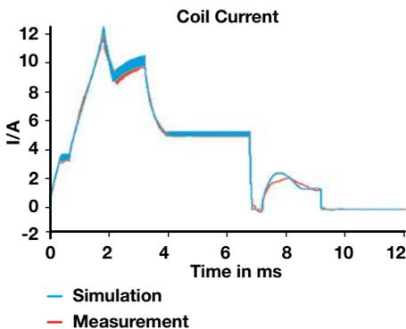
**Figure 8** Comparison of measurement and simulation results
